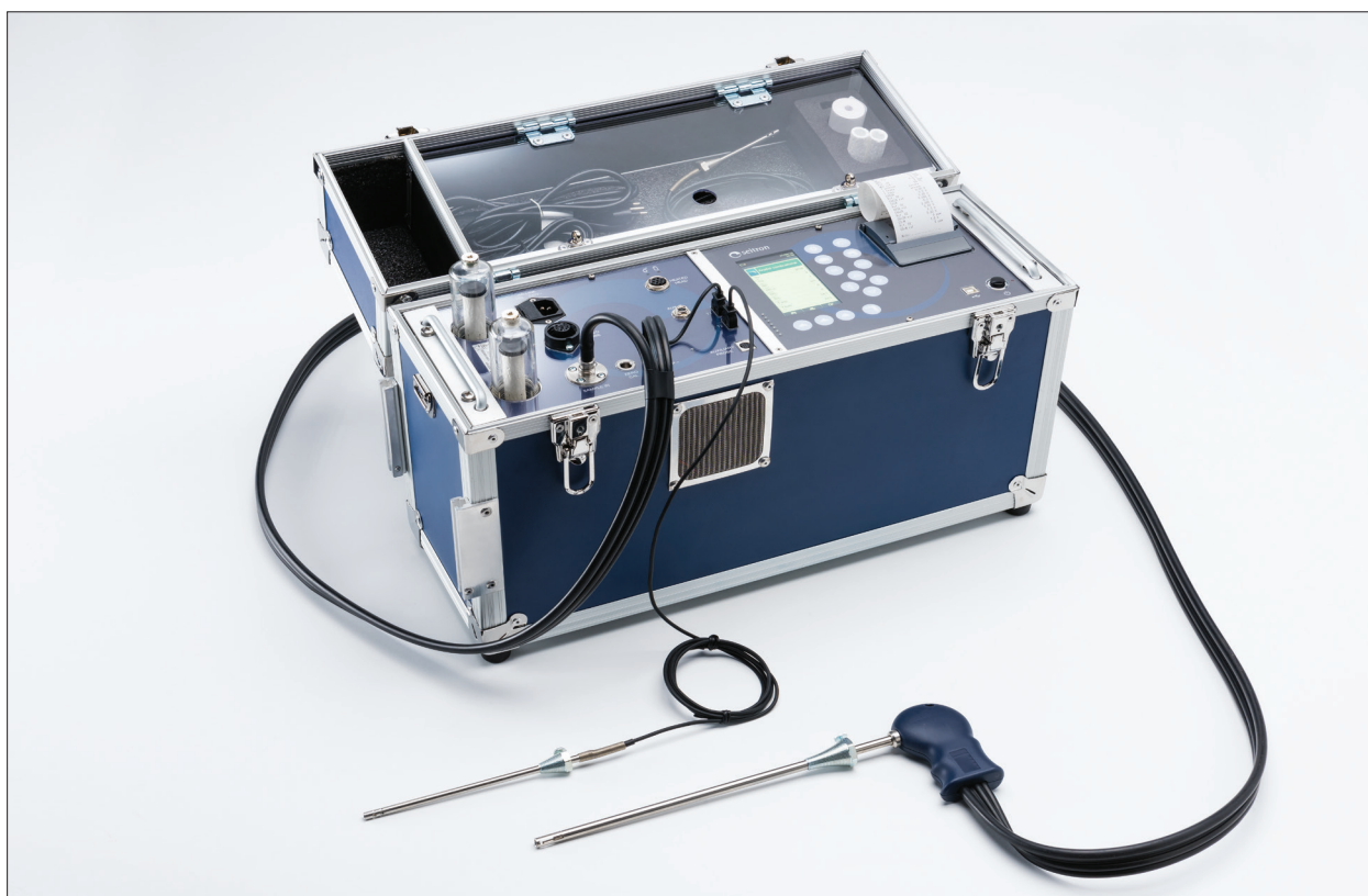
Chemist 900 with active heated gas sampling probe
