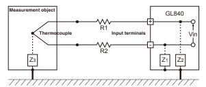
Connect the signal chassis GND to the measurement device chassis ground.
