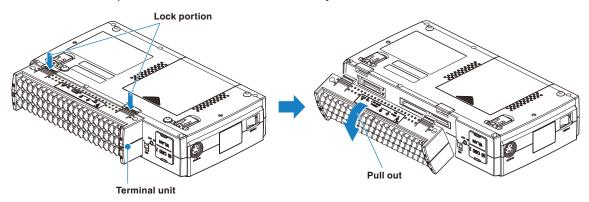
(2) Pull the terminal unit out towards the direction indicated by the arrow.
