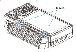
(2) Press the terminal unit in the direction shown until it is securely locked.
