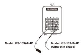
No. 1 to 4 is the thermistor connection terminal.
