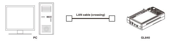
• Use a straight cable when using a hub.
