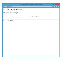
To display the FTP site in the Explorer from the figure above, press the Alt key and click the "View" and then click the "Open FTP site with Explorer". The foillowing screen is displayed.
