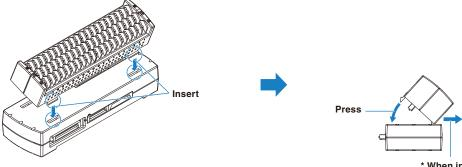
\* When installing the Withstand highvoltage high-precision terminal (B-565), please push it while pulling to the front.
