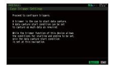
3. After setting, when you the "Next>>" is selected and then the [ENTER] key is pressed, the "Sampling, Interval, Capture Destination" screens are displayed. Set the necessary items.
