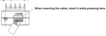
No. 1 to 4: High-voltage terminal (terminal input on the input signal's high-voltage side)
