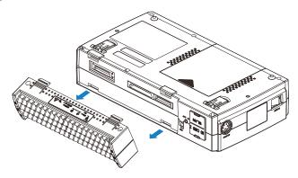
Pull the terminal unit out as shown in the following figure.
