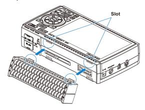
(1) Insert tabs at the top of the terminal unit into the slots.
