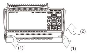
(3) When both corners of rubber protector are removed from the body, remove the body completely from the rubber protector.
