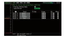
This is used to perform the setting related to the digital input to the GL840.
