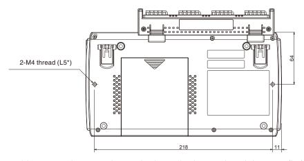
\* When rubber protection cover is attached, required screw length is 8 mm (L8).
