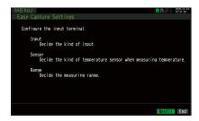
2. When the settings (input, sensor, and range) are satisfied, select the "Next>>" and then press the [ENTER] key. The "Input, Sensor, and Range, etc." screens are displayed. Set the necessary items.
