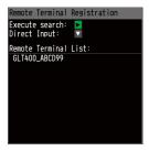
Then, when the unit name to be connected is selected from the displayed remote sensor list, the unit name is automatically registered.
