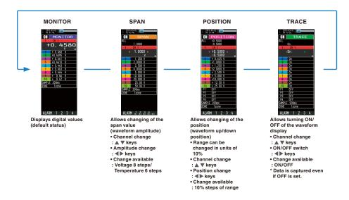
\* When ALL is set, setting values for CH1 is reflected on other channels. When CH1 is OFF, ALL cannot be set.
