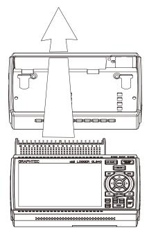
(2) While opening the rubber protector slightly, put the body in it.
