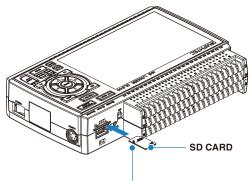
\* Make sure that the SD CARD is not locked.
