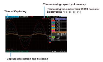
The captured data is saved in the internal memory (SD1) or SD CARD (SD2) during data capture. You cannot use the [MENU] key to change the setting.
