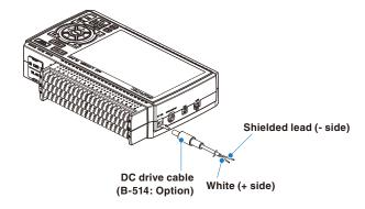
(3) Connect the DC input side to the DC power supply.
