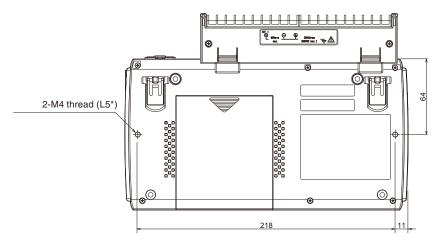
\* When rubber protection cover is attached, required screw length is 8 mm (L8).
