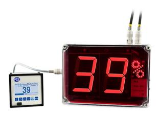
PCE-G1A is an environmental meter with a large display. This IP54-rated wall-mountable device measures both relative humidity (%RH) and temperature (°C only). The PCE-G1A environmental meter has a large LED display with a number height of 100 mm / 3.9 in, so measurement values can be seen at a distance of up to 50 m / 164 ft away.
