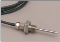
ES-325 Screw-In Probe For air and water temperature D=4mm, L=30mm M8 outside thread
