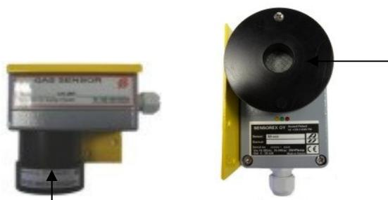
2. Set the Gas-In nipple to the hole of the adapter.
