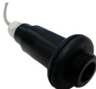
Drill a 34mm hole to the duct in a place where the monitoring is wanted. For correct measurement, the hole should be drilled on the top of the duct. This also prevents the possibly condensing water from flowing into the sensor element. Install the rubber gasket to the hole.
