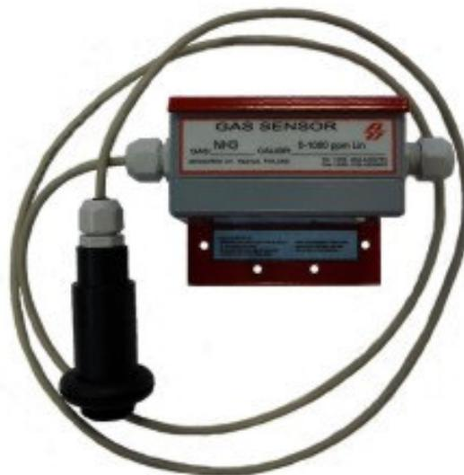
Duct version of the sensor includes the same mounting bracket and enclosure as normal one without the black sensor cover. The sensing element itself is inside the adapter which is delivered with 1,5 meter (standard) cable and is intended to be installed to a duct with a rubber gasket, also delivered with the sensor.
