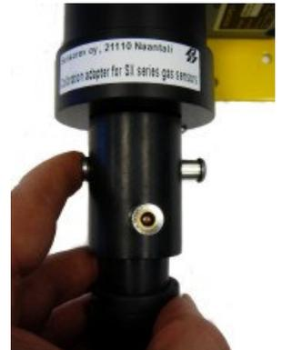
7. After successful calibration, first remove the adapter (+ calibration bag + valve) and then close the valve.
