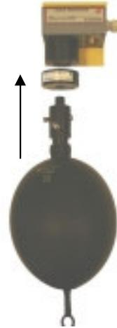
5. Open the valve of the bag and gently squeeze the bag in order to get a steady gas flow.
