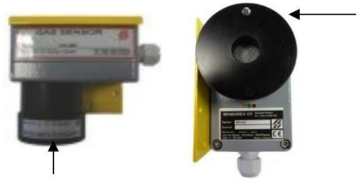
2. Set the Gas-In nipple to the hole of the adapter.
