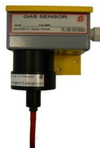
3. Attach a hose between calibration gas cylinder's valve and the Gas-In nipple.
