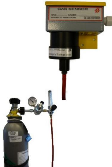
5. Check the result by measuring the sensor output signal or checking from possible monitor value after the reading is stable.
