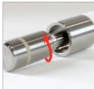
3. Unscrew the HiTemp140-M12 data logger, from the lid of the thermal barrier.
