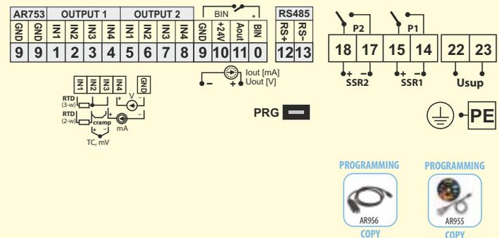
PRG - programmer connector is available after unscrewing cap in the left side of the housing (next to the keyboard). (do not use simultaneously with RS485)
