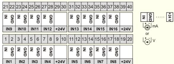
c) 8 pulse inputs version, INPUT1 ÷ INPUT8
