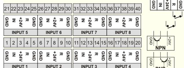
d) 4 universal and 4 pulse inputs version, INPUT1 ÷ INPUT8
