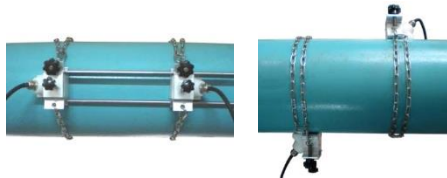
M-Mounting Frame (V method and Z method)
