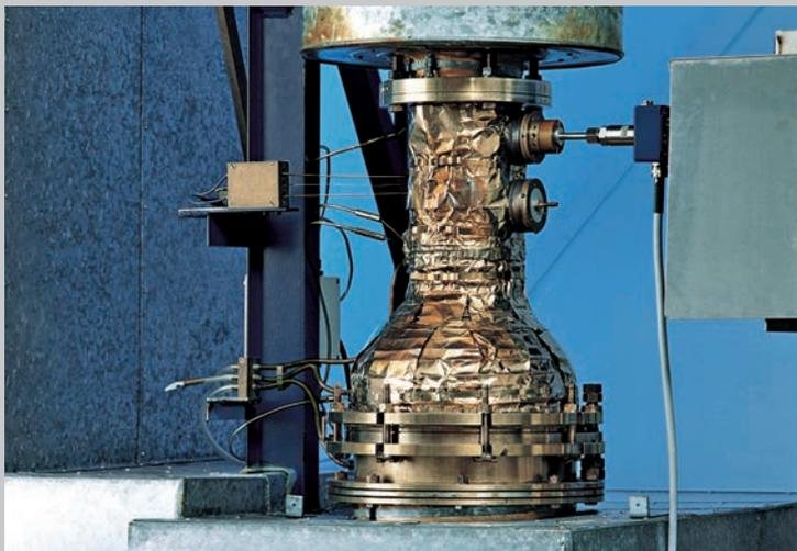
**High temperature wind tunnel, 0.1 ... 80 m/s, +20 °C... +400 °C**
