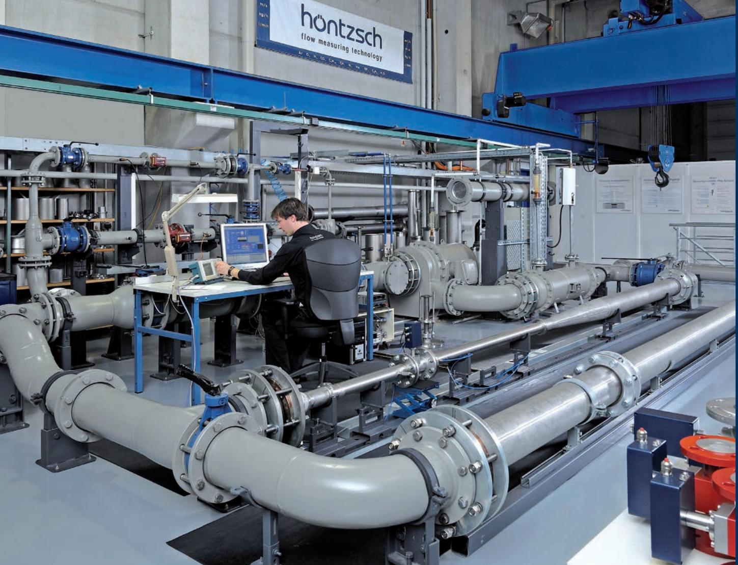
**Volume flow calibration installation, pressure up to 10 bar, 1 MPa, nominal value up to DN200**
